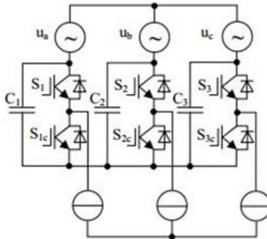
Fig.2 Three-phase differential AC chopper.
