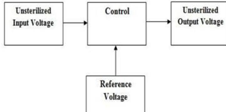
*Fig 1 Block Diagram of Voltage Stabilizer*
